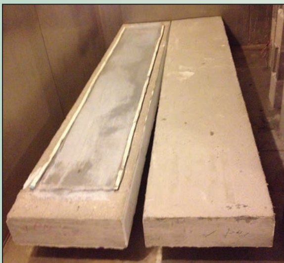
Figure 1. Strengthened slabs inside the environmental chamber at Missouri S&T
